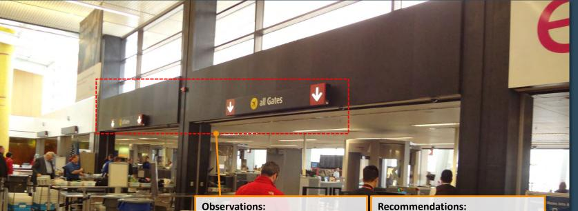
**1. Scale:** Existing soffit directionals appear out of scale/too small **2. Illumination:** Inconsistent use of illumination on directionals
